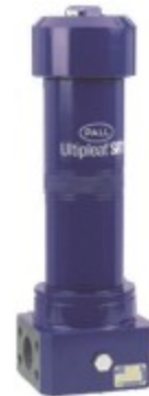
Up319 Series High Pressure Filters Equivalent Flows to 600 L/min (160 US gpm) Pressures to 250 bard (3625 psid) Port size 1/4", 1/2" and 2" Patented Utlpleat (laid-over pleat) filter medium pack Coreless, cageless element configuration Pall Stress-Resistant Technology (SRT) Media In-to-out filter element flow path
