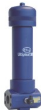
Pall UH319 Series Filters Equivalent In-to-out filter element flow path Flows to 600 L/min (160 US gpm) Pressures to 420 bar (6100 psi) Ports, 1 1/2" top and side manifold mount Coreless, cageless element configuration
