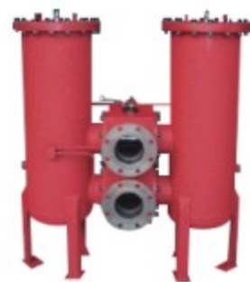
Hydac RFLD Series Change-Over Inline Filter Equivalent Nominal pressure: 16 bar Temperature range: -10 °C to +100 °C Connection: DN 40-DN 300 Flow rate: 15000 l/min
