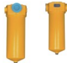
ZU-A QU-A WU-A XU-A Return Line Filter Series Flow rate: 10-630L/min Pressure: 1.6 MPa Precision: 1-30µm Dia.: 10-65mm Connecting: Thread, Flange Element Model: TZX2 Series
