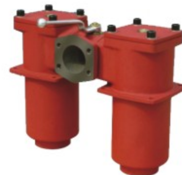
Up319 Series High Pressure Filters Equivalent Flows to 600 L/min (160 US gpm) Pressures to 250 bard (3625 psid) Port size 1/4", 1/2" and 2" Patented Utlpleat (laid-over pleat) filter medium pack Coreless, cageless element configuration Pall Stress-Resistant Technology (SRT) Media In-to-out filter element flow path
