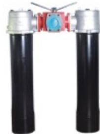
SRFB Duplex Tank Mounted Return Filter Series Flow rate: 25-1300L/min Pressure: 1.6 MPa Precision: 1-30µm Dia.: 50mm 80mm Connecting: Flange Element Model: SFBX Serie
