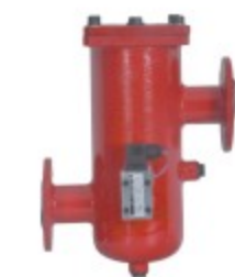
RLF Return Line Filter Series Flow rate: 60-1300L/min Pressure: 1.6MPa Precision: 1-20µm Dia.: 25-100mm Connecting: Flange Element Model: SFX Series
