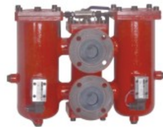
SRLF Duplex Return Line Filter Series Flow rate: 60-1300L/min Pressure: 1.6 MPa Precision: 1-30µm Dia.: 25-100mm Connecting: Flange Element Model: SFX Series
