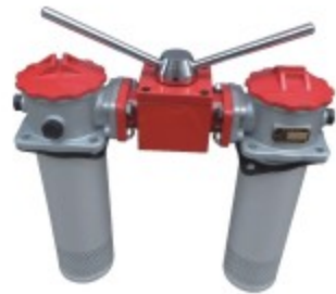
SRFA Duplex Tank Mounted Mini-type Return Filter Series Flow rate: 25-1000L/min Pressure: 1.6 MPa Precision: 1-30µm Dia.: 20-90mm Connecting: Screw, Flange Element Model: SFX Series
