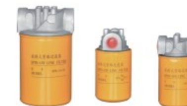
Spin Line Filter Flow rate: suction: 25-80L/min return: 60-320L/min Maximum Pressure: 0.7MPa Precision: 1-30µm Connecting: Thread Element Model: SP (A, B) X Series
