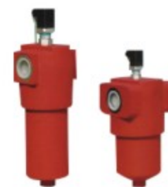
Hydac DF Series Pressure Filter Equivalent Nominal pressure: 260 bar Bypass cracking pressure : 6 bar Temperature: -10 °C to +100 °C Connection: Flow rate : 500L/min
